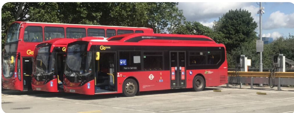
Bus2Grid project demonstrating electric buses at Northumberland Garage in North London connected to vehicle-to-grid chargers
